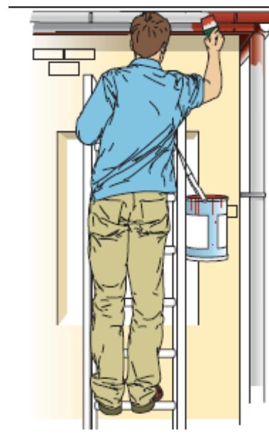
Maintaining 3 points of contact
