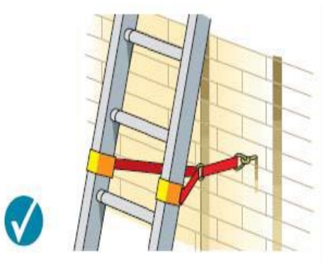
Tying near the base
